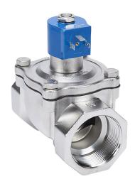
GC Valves potable water solenoid valve, 2-port (2-way), 2-position, N.C., 316 stainless steel body, 2in female NPT inlet(s), 2in female NPT outlet(s), Cv=28, 120 VAC (60Hz)/110 VAC (50Hz) operating voltage, 8W, NSF/ANSI/CAN 61.
