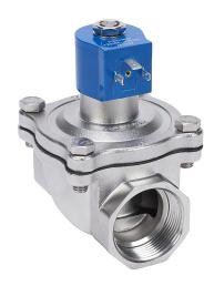
GC Valves potable water solenoid valve, 2-port (2-way), 2-position, N.C., 316 stainless steel body, 1-1/2in female NPT inlet(s), 1-1/2in female NPT outlet(s), Cv=13, 120 VAC (60Hz)/110 VAC (50Hz) operating voltage, 8W, NSF/ANSI/CAN 61.
