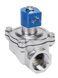
GC Valves potable water solenoid valve, 2-port (2-way), 2-position, N.C., 316 stainless steel body, 1-1/4in female NPT inlet(s), 1-1/4in female NPT outlet(s), Cv=13, 120 VAC (60Hz)/110 VAC (50Hz) operating voltage, 8W, NSF/ANSI/CAN 61.
