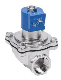
GC Valves potable water solenoid valve, 2-port (2-way), 2-position, N.C., 316 stainless steel body, 1in female NPT inlet(s), 1in female NPT outlet(s), Cv=13, 120 VAC (60Hz)/110 VAC (50Hz) operating voltage, 8W, NSF/ANSI/CAN 61.
