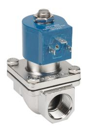
GC Valves potable water solenoid valve, 2-port (2-way), 2-position, N.C., 316 stainless steel body, 3/4in female NPT inlet(s), 3/4in female NPT outlet(s), Cv=6.7, 120/110 VAC operating voltage, 8W, NSF/ANSI/CAN 61.
