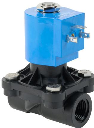
GC Valves potable water solenoid valve, 2-port (2-way), 2-position, N.C., Nylon 6 body, 1/2in female NPT inlet(s), 1/2in female NPT outlet(s), Cv=4.3, 24 VAC operating voltage, 10W, NSF/ANSI/CAN 61.
