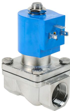
GC Valves potable water solenoid valve, 2-port (2-way), 2-position, N.C., 316 stainless steel body, 3/4in female NPT inlet(s), 3/4in female NPT outlet(s), Cv=6.7, 24 VAC operating voltage, 10W, NSF/ANSI/CAN 61.
