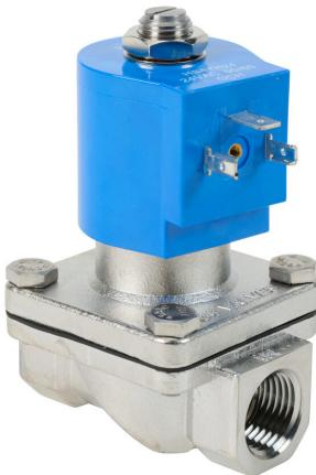
GC Valves potable water solenoid valve, 2-port (2-way), 2-position, N.C., 316 stainless steel body, 1/2in female NPT inlet(s), 1/2in female NPT outlet(s), Cv=4.3, 24 VAC operating voltage, 10W, NSF/ANSI/CAN 61.
