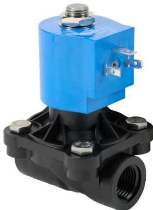
GC Valves potable water solenoid valve, 2-port (2-way), 2-position, N.C., Nylon 6 body, 1/2in female NPT inlet(s), 1/2in female NPT outlet(s), Cv=4.3, 24 VDC operating voltage, 10W, NSF/ANSI/CAN 61.
