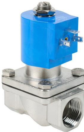
GC Valves potable water solenoid valve, 2-port (2-way), 2-position, N.C., 316 stainless steel body, 3/4in female NPT inlet(s), 3/4in female NPT outlet(s), Cv=6.7, 24 VDC operating voltage, 10W, NSF/ANSI/CAN 61.
