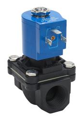
GC Valves potable water solenoid valve, 2-port (2-way), 2-position, N.C., Nylon 6 body, 3/4in female NPT inlet(s), 3/4in female NPT outlet(s), Cv=6.7, 24 VAC operating voltage, 10W.
