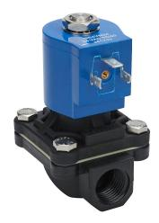
GC Valves potable water solenoid valve, 2-port (2-way), 2-position, N.C., Nylon 6 body, 1/2in female NPT inlet(s), 1/2in female NPT outlet(s), Cv=4.3, 24 VAC operating voltage, 10W.
