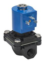
GC Valves potable water solenoid valve, 2-port (2-way), 2-position, N.C., Nylon 6 body, 3/8in female NPT inlet(s), 3/8in female NPT outlet(s), Cv=4.3, 24 VAC operating voltage, 10W.
