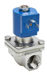
GC Valves potable water solenoid valve, 2-port (2-way), 2-position, N.C., 316 stainless steel body, 3/4in female NPT inlet(s), 3/4in female NPT outlet(s), Cv=6.7, 24 VAC operating voltage, 10W.
