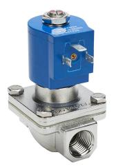
GC Valves potable water solenoid valve, 2-port (2-way), 2-position, N.C., 316 stainless steel body, 1/2in female NPT inlet(s), 1/2in female NPT outlet(s), Cv=4.3, 24 VAC operating voltage, 10W.
