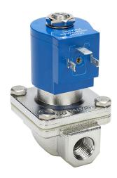
GC Valves potable water solenoid valve, 2-port (2-way), 2-position, N.C., 316 stainless steel body, 3/8in female NPT inlet(s), 3/8in female NPT outlet(s), Cv=4.3, 24 VAC operating voltage, 10W.
