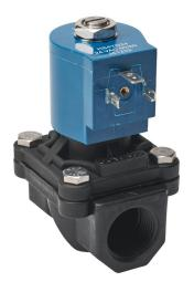
GC Valves potable water solenoid valve, 2-port (2-way), 2-position, N.C., Nylon 6 body, 3/4in female NPT inlet(s), 3/4in female NPT outlet(s), Cv=6.7, 24 VAC operating voltage, 10W, NSF/ANSI/CAN 61.
