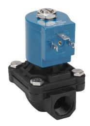
GC Valves potable water solenoid valve, 2-port (2-way), 2-position, N.C., Nylon 6 body, 1/2in female NPT inlet(s), 1/2in female NPT outlet(s), Cv=4.3, 24 VAC operating voltage, 10W, NSF/ANSI/CAN 61.
