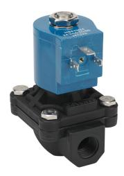
GC Valves potable water solenoid valve, 2-port (2-way), 2-position, N.C., Nylon 6 body, 3/8in female NPT inlet(s), 3/8in female NPT outlet(s), Cv=4.3, 24 VAC operating voltage, 10W, NSF/ANSI/CAN 61.
