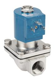
GC Valves potable water solenoid valve, 2-port (2-way), 2-position, N.C., 316 stainless steel body, 1/2in female NPT inlet(s), 1/2in female NPT outlet(s), Cv=4.3, 24 VAC operating voltage, 10W, NSF/ANSI/CAN 61.
