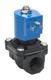
GC Valves potable water solenoid valve, 2-port (2-way), 2-position, N.C., Nylon 6 body, 3/4in female NPT inlet(s), 3/4in female NPT outlet(s), Cv=6.7, 24 VDC operating voltage, 10W.
