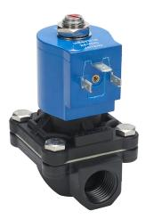
GC Valves potable water solenoid valve, 2-port (2-way), 2-position, N.C., Nylon 6 body, 1/2in female NPT inlet(s), 1/2in female NPT outlet(s), Cv=4.3, 24 VDC operating voltage, 10W.
