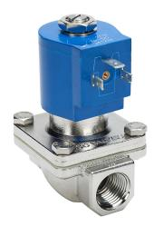
GC Valves potable water solenoid valve, 2-port (2-way), 2-position, N.C., 316 stainless steel body, 1/2in female NPT inlet(s), 1/2in female NPT outlet(s), Cv=4.3, 24 VDC operating voltage, 10W.
