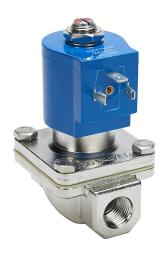
GC Valves potable water solenoid valve, 2-port (2-way), 2-position, N.C., 316 stainless steel body, 3/8in female NPT inlet(s), 3/8in female NPT outlet(s), Cv=4.3, 24 VDC operating voltage, 10W.
