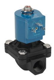
GC Valves potable water solenoid valve, 2-port (2-way), 2-position, N.C., Nylon 6 body, 1/2in female NPT inlet(s), 1/2in female NPT outlet(s), Cv=4.3, 24 VDC operating voltage, 10W, NSF/ANSI/CAN 61.
