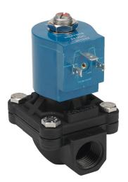
GC Valves potable water solenoid valve, 2-port (2-way), 2-position, N.C., Nylon 6 body, 1/2in female NPT inlet(s), 1/2in female NPT outlet(s), Cv=4.3, 24 VDC operating voltage, 10W, NSF/ANSI/CAN 61.
