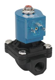
GC Valves potable water solenoid valve, 2-port (2-way), 2-position, N.C., Nylon 6 body, 3/8in female NPT inlet(s), 3/8in female NPT outlet(s), Cv=4.3, 24 VDC operating voltage, 10W, NSF/ANSI/CAN 61.
