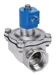
GC Valves potable water solenoid valve, 2-port (2-way), 2-position, N.C., 316 stainless steel body, 1-1/2in female NPT inlet(s), 1-1/2in female NPT outlet(s), Cv=18, 24 VDC operating voltage, 10W, NSF/ANSI/CAN 61.
