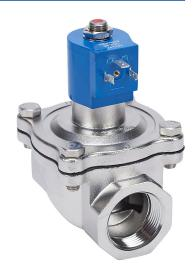
GC Valves potable water solenoid valve, 2-port (2-way), 2-position, N.C., 316 stainless steel body, 1-1/4in female NPT inlet(s), 1-1/4in female NPT outlet(s), Cv=18, 24 VDC operating voltage, 10W, NSF/ANSI/CAN 61.
