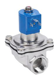
GC Valves potable water solenoid valve, 2-port (2-way), 2-position, N.C., 316 stainless steel body, 1in female NPT inlet(s), 1in female NPT outlet(s), Cv=11, 24 VDC operating voltage, 10W, NSF/ANSI/CAN 61.
