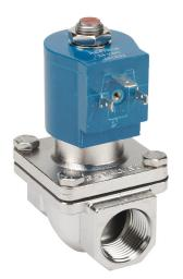
GC Valves potable water solenoid valve, 2-port (2-way), 2-position, N.C., 316 stainless steel body, 3/4in female NPT inlet(s), 3/4in female NPT outlet(s), Cv=6.7, 24 VDC operating voltage, 10W, NSF/ANSI/CAN 61.
