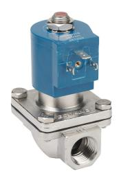
GC Valves potable water solenoid valve, 2-port (2-way), 2-position, N.C., 316 stainless steel body, 1/2in female NPT inlet(s), 1/2in female NPT outlet(s), Cv=4.3, 24 VDC operating voltage, 10W, NSF/ANSI/CAN 61.
