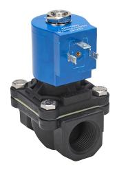
GC Valves potable water solenoid valve, 2-port (2-way), 2-position, N.C., Nylon 6 body, 3/4in female NPT inlet(s), 3/4in female NPT outlet(s), Cv=6.7, 120/110 VAC operating voltage, 10W.
