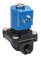
GC Valves potable water solenoid valve, 2-port (2-way), 2-position, N.C., Nylon 6 body, 1/2in female NPT inlet(s), 1/2in female NPT outlet(s), Cv=4.3, 120/110 VAC operating voltage, 10W.
