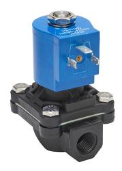
GC Valves potable water solenoid valve, 2-port (2-way), 2-position, N.C., Nylon 6 body, 3/8in female NPT inlet(s), 3/8in female NPT outlet(s), Cv=4.3, 120/110 VAC operating voltage, 10W
