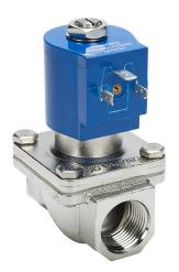
GC Valves potable water solenoid valve, 2-port (2-way), 2-position, N.C., 316 stainless steel body, 3/4in female NPT inlet(s), 3/4in female NPT outlet(s), Cv=6.7, 120/110 VAC operating voltage, 10W.
