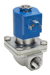
GC Valves potable water solenoid valve, 2-port (2-way), 2-position, N.C., 316 stainless steel body, 1/2in female NPT inlet(s), 1/2in female NPT outlet(s), Cv=4.3, 120/110 VAC operating voltage, 10W.
