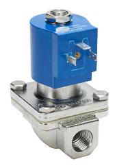
GC Valves potable water solenoid valve, 2-port (2-way), 2-position, N.C., 316 stainless steel body, 3/8in female NPT inlet(s), 3/8in female NPT outlet(s), Cv=4.3, 120/110 VAC operating voltage, 10W.
