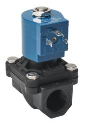
GC Valves potable water solenoid valve, 2-port (2-way), 2-position, N.C., Nylon 6 body, 3/4in female NPT inlet(s), 3/4in female NPT outlet(s), Cv=6.7, 120/110 VAC operating voltage, 10W, NSF/ANSI/CAN 61.
