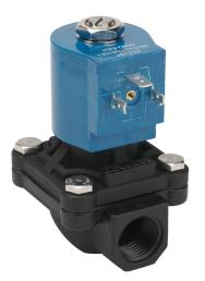
GC Valves potable water solenoid valve, 2-port (2-way), 2-position, N.C., Nylon 6 body, 1/2in female NPT inlet(s), 1/2in female NPT outlet(s), Cv=4.3, 120/110 VAC operating voltage, 10W, NSF/ANSI/CAN 61.
