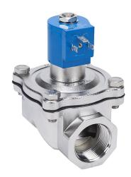
GC Valves potable water solenoid valve, 2-port (2-way), 2-position, N.C., 316 stainless steel body, 1-1/4in female NPT inlet(s), 1-1/4in female NPT outlet(s), Cv=18, 120 VAC (60Hz)/110 VAC (50Hz) operating voltage, 10W, NSF/ANSI/CAN 61.
