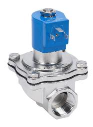
GC Valves potable water solenoid valve, 2-port (2-way), 2-position, N.C., 316 stainless steel body, 1in female NPT inlet(s), 1in female NPT outlet(s), Cv=11, 120 VAC (60Hz)/110 VAC (50Hz) operating voltage, 10W, NSF/ANSI/CAN 61.
