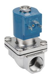
GC Valves potable water solenoid valve, 2-port (2-way), 2-position, N.C., 316 stainless steel body, 3/4in female NPT inlet(s), 3/4in female NPT outlet(s), Cv=6.7, 120/110 VAC operating voltage, 10W, NSF/ANSI/CAN 61.
