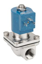
GC Valves potable water solenoid valve, 2-port (2-way), 2-position, N.C., 316 stainless steel body, 1/2in female NPT inlet(s), 1/2in female NPT outlet(s), Cv=4.3, 120/110 VAC operating voltage, 10W, NSF/ANSI/CAN 61.
