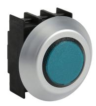
Schmersal illuminated indicating light, permanent light function, IP67 and IP69K, 22mm, green, 44mm, round, plastic base, plastic bezel. Requires light block and LED or incandescent bulb.
