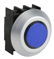
Schmersal illuminated indicating light, permanent light function, IP67 and IP69K, 22mm, blue, 44mm, round, plastic base, plastic bezel. Requires light block and LED or incandescent bulb.
