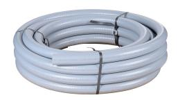
Electri-Flex Liquatite liquid-tight flexible non-metalic conduit, embedded spiral rigid PVC, PVC wall, 1-1/2in trade size, gray, UL-1660 Listed, 50ft/15.2m coil length.
