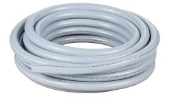
Electri-Flex Liquatite liquid-tight flexible non-metalic conduit, embedded spiral rigid PVC, PVC wall, 1in trade size, gray, UL-1660 Listed, 50ft/15.2m coil length.
