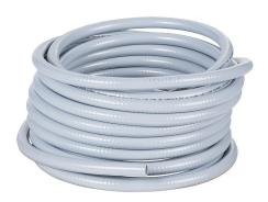
Electri-Flex Liquatite liquid-tight flexible non-metalic conduit, embedded spiral rigid PVC, PVC wall, 1/2in trade size, gray, UL-1660 Listed, 50ft/15.2m coil length.
