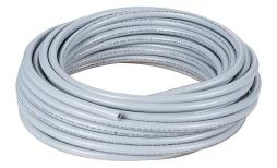
Electri-Flex Liquatite liquid-tight flexible non-metalic conduit, embedded spiral rigid PVC, PVC wall, 3/8in trade size, gray, UL-1660 Listed, 100ft/30.4m coil length.
