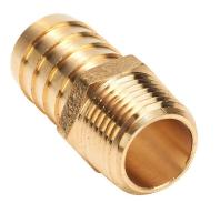
HydroMode threaded fitting, hose barb, lead-free brass body, lead-free brass threads, (1) 3/4in hose to (1) 1/2in male NPT connection(s). Package of 3.
